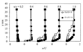
Fig. 5 Effect of leading-edge rotating cylinder on velocity profiles on the upper surface of the airfoil.
