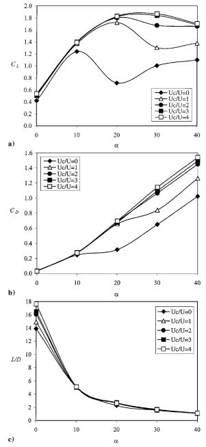
Fig. 3 Effect of plain flap at  $\delta = 30 \deg \text{ on a}$  lift coefficient  $C_L$ , b) drag coefficient  $C_D$ , and c) lift-to-drag ratio L/D.
