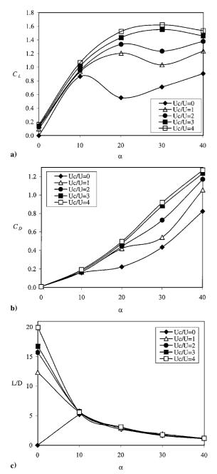
Fig. 2 Effect of leading-edge rotating cylinder at  $\delta = 0$  on a) lift coefficient  $C_L$ , b) drag coefficient  $C_D$ , and c) lift-to-drag ratio L/D.
